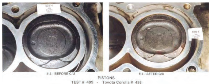
Picture G - Piston before P.i. treatment
